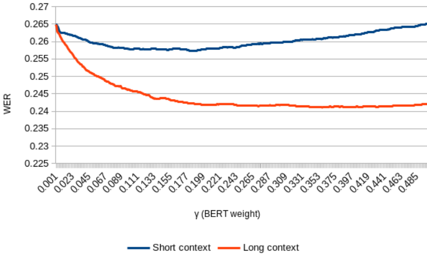
Figure 6.1: WER on the NPSC evaluation set with 2 and 5 context utterances available to BERT when rescoring. It is clear that longer context improves results on this dataset.
